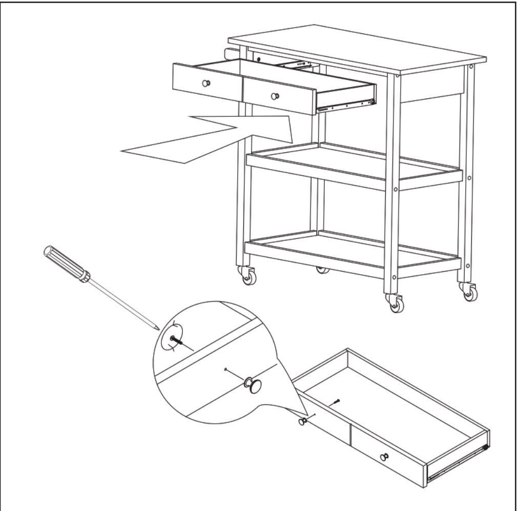
Step 6 : Attach the silver metal knob, then insert the drawer unit through the slider rail.
