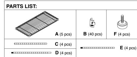
Snap sleeves (B) into the grooves on the lower bottom of the four legs, slide the first shelf onto the 4 sleeves from the four poles, using a rubbermallet gently pounds to a tight fit
