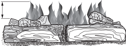
Figure 32 - Correct Burner Flame Pattern
