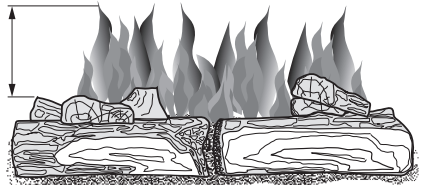
Figure 33 - Incorrect Burner Flame Pattern
