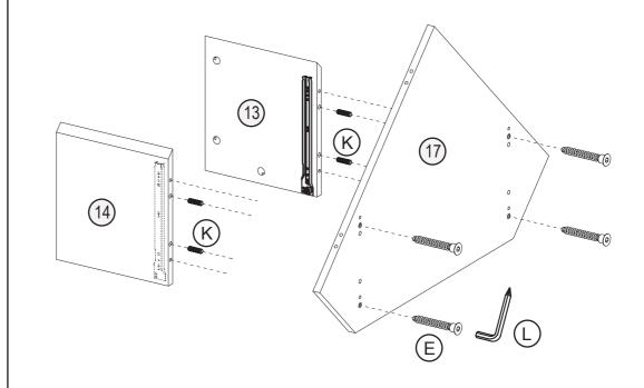
Attach cam bolts to the shelf panel (17). 8 M6 x 35mm (17) A 4x K Ø8 x 30mm Ø A K 4x 9
