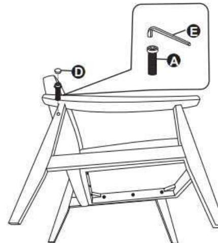
Put the screws in the holes, tight the screws, but not too tight, 90% is ok.
