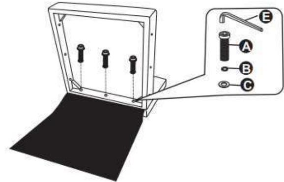
Put the screws in the holes, tight the screws, but not too tight, 90% is ok.
