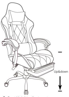
2 Seat Height adjustment (pull up on the control handle to adjust)
