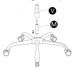
4 . Fix the control unit to the base of the seat
