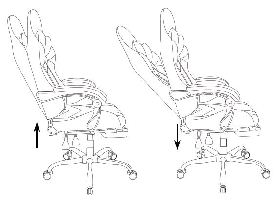
pull up on the rear control handle to adjust the reclining angle
