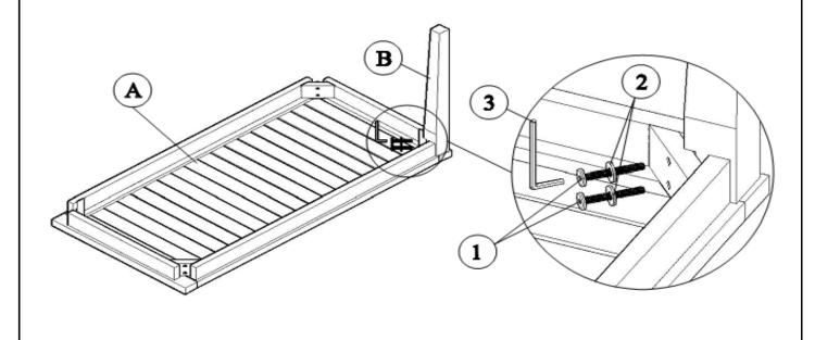
Attach Leg(B) to Table Top(A) using Bolts( $\widehat{1}$ ) and Washers( $\widehat{2}$ ) with Allen Wrench( $\widehat{3}$ ) as shown above.
