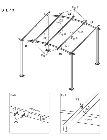
Fig.6: Using Bolt (AA) to connect Roof Tubes (D1 &D2).
