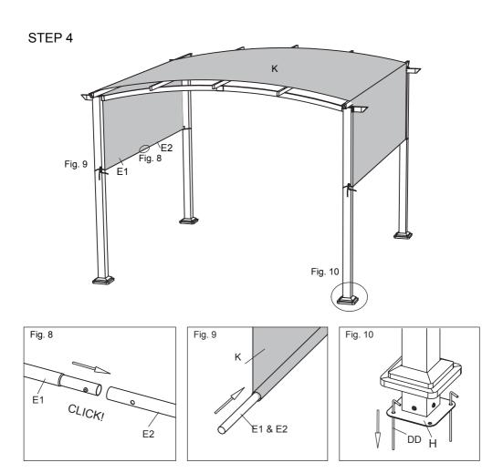
Fig.8: Insert Weight Bar (E1) to Weight Bar (E2) till you will see the push pin out from the tube. Fig.9: Pass the Shade Fabric K through the Roof Tube (D1/D2) in turn as above diagram. Make sure Cross Beam (C1/C2) on the edge support the Shade Fabric underneath. Insert the Pulling Rod (E1/E2) to Shade Fabric. After assembled, please pull the Shade Fabric, make sure it runs smoothly.
