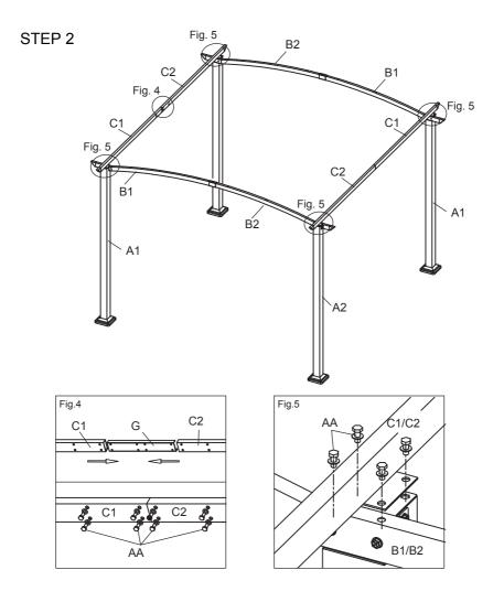
Fig.4: Insert Connector Tube (G) to Lintel (C1) and Lintel (C2), make sure the holes are aligned. Then use Bolt (AA) to connect Lintel (C1), Lintel (C2) and Connector Tube (G). Fig.5: Using Bolt (AA) to connect Lintel (C1) and Roof Tube Curved (B1). Using Bolt (AA)
