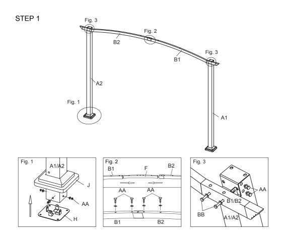
Fig.1: Insert Post(A1) to Base Plate Cover (J), then using Bolt (AA) to connect Post (A1 & A2) and Base Plate (H). Repeat each step for A1/A2.
