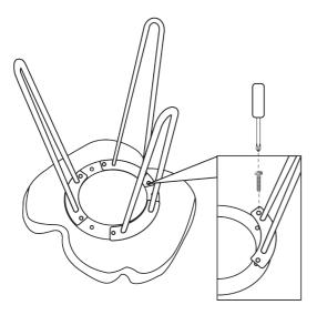
Attach the legs with the screws provided. Please note that the screws provided are the proper length for 1.5" to 2" thick.
