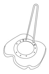
Line up one leg at a time to the holes in the mounting plate.
