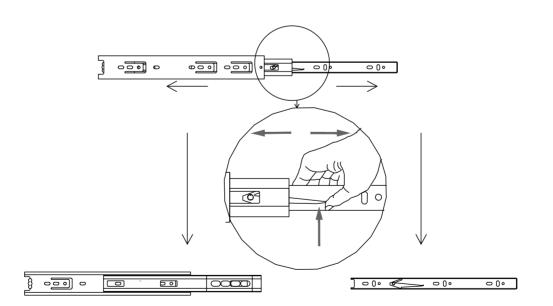
Disconnect the rail with the BLACK PLASTIC PART. It needs to be pulled down to disconnect the runners.
