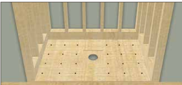
Step5: Plywood Sub-Floor
