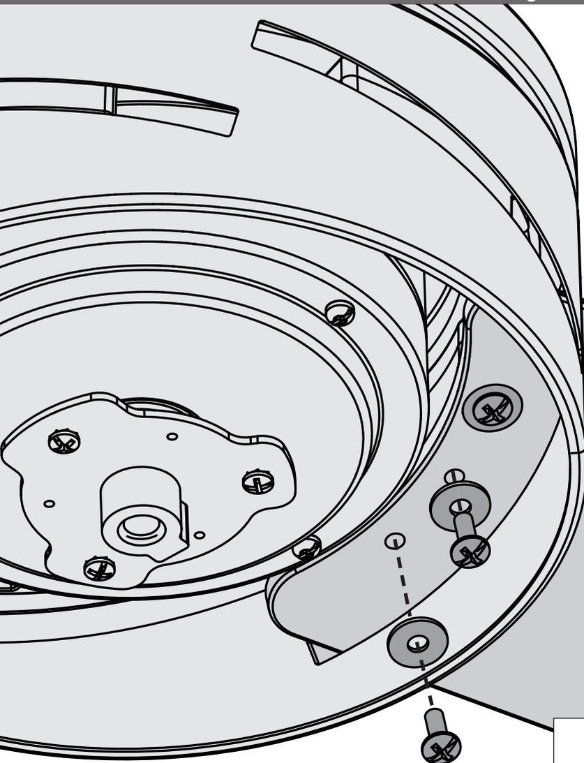
Put the blade washers found in the ■ hardware bag onto the blade screws found in the ▲ hardware bag. Then install the blade screws to secure each blade to the fan.
