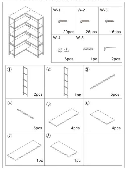
**Notes:** Don't tighten screws completely at first, just in case parts were assembled wrong and need disassembled. Tighten screws at last when all parts are put together.
