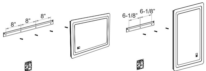
**Note:** Ideal distance of drill holes for mirror orientation
