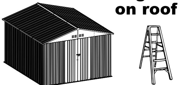
NEVER concentrate your weight on the roof of the building. When using a step ladder make sure that it is fully open and on even ground before climbing on it.
