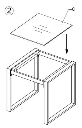
Do not tight all screws before assemble completely
