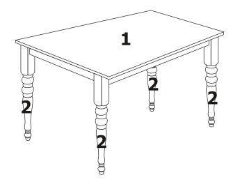
Place the Table Top(1) bottom-side up on a clean and soft surface. Attach individual Table Leg(2) using JCBB Bolts(A), inserted with Spring Washer(C) and Flat Washer(B). Tighten with Allen Key(D). Do not over-tighten JCBB Bolts(A). Turn table right-side up with the help of another person.
