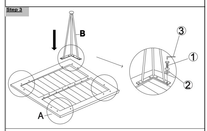
Insert leg (B) into the table top  $\,$  (A), put the flat washers ( $\,$  ② $\,$ ) and bolt ( $\,$ 0 $\,$ ) as above picture.
