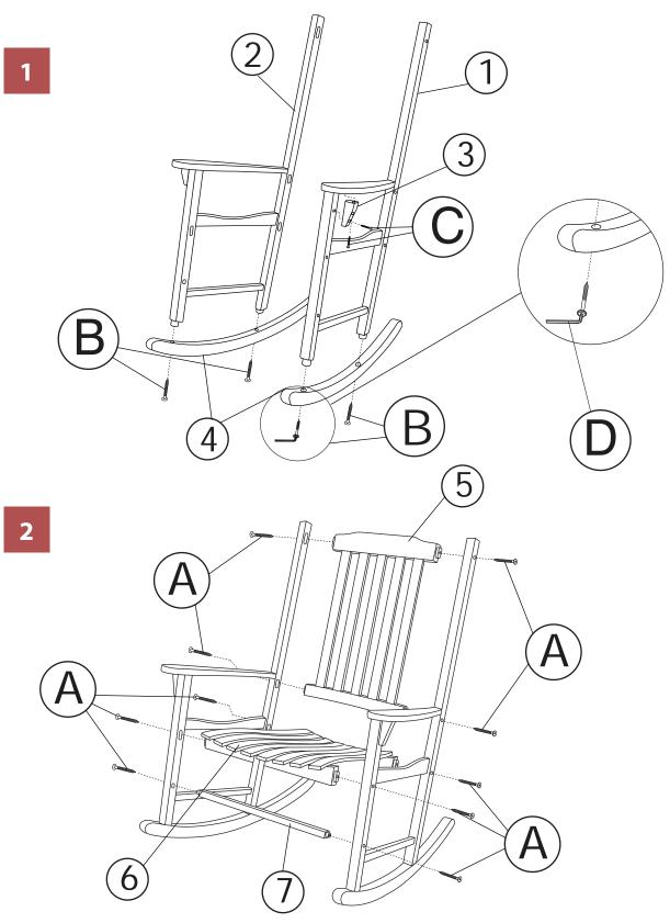
NOTE: Please read all instructions carefully before starting assembly. Also, we recommend that the unit is fully assembled on a level surface. Two people are recommended to assemble this product. DO NOT over torque screws and bolts.
