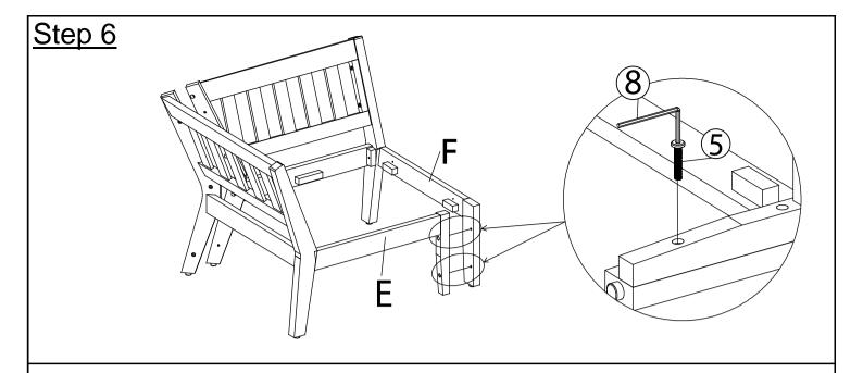
Align the Left Panel(E) to Right Panel(H) and attach using Bolts( $\overline{\$}$ ) with Allen Key( $\overline{\$}$ ). **Do not fully tighten the Bolts.**
