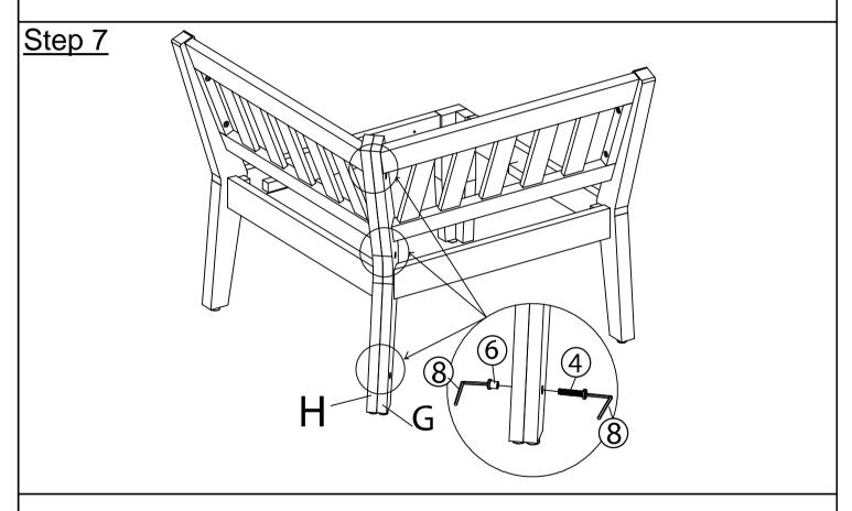
Align Left Corner Leg(G) to Right Corner Leg(H) as shown above. Attach Left Corner Leg(G) to Right Corner Leg(H) using Bolts(4) and Sleeve Nuts(6) with Allen Keys(8).
