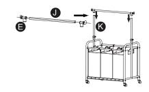
STEP 7. Put two ends of Hanging Bar (J) into the hole of Top Plastic Joint (E) and keep another hole vertically downward, then insert them into the upright bar (K).
