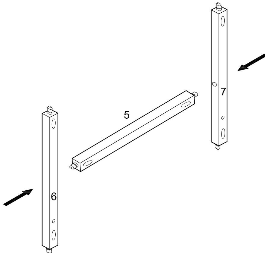
Attach crossbars (6,7) to crossbar (5) using dowels as guides.
