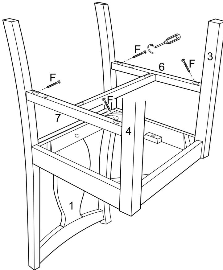
Secure crossbars (6,7) to chair legs (3,4) and chair back (1) using screws (F). Tighten screws (F) with a screwdriver.
