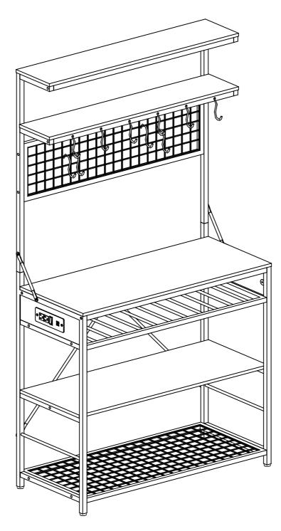
**GAUTION**: When tightening the screws, tighten sequentially. Do not tighten any screws fully and then towards the next one. When every part is OK, then tighten all the screws.
