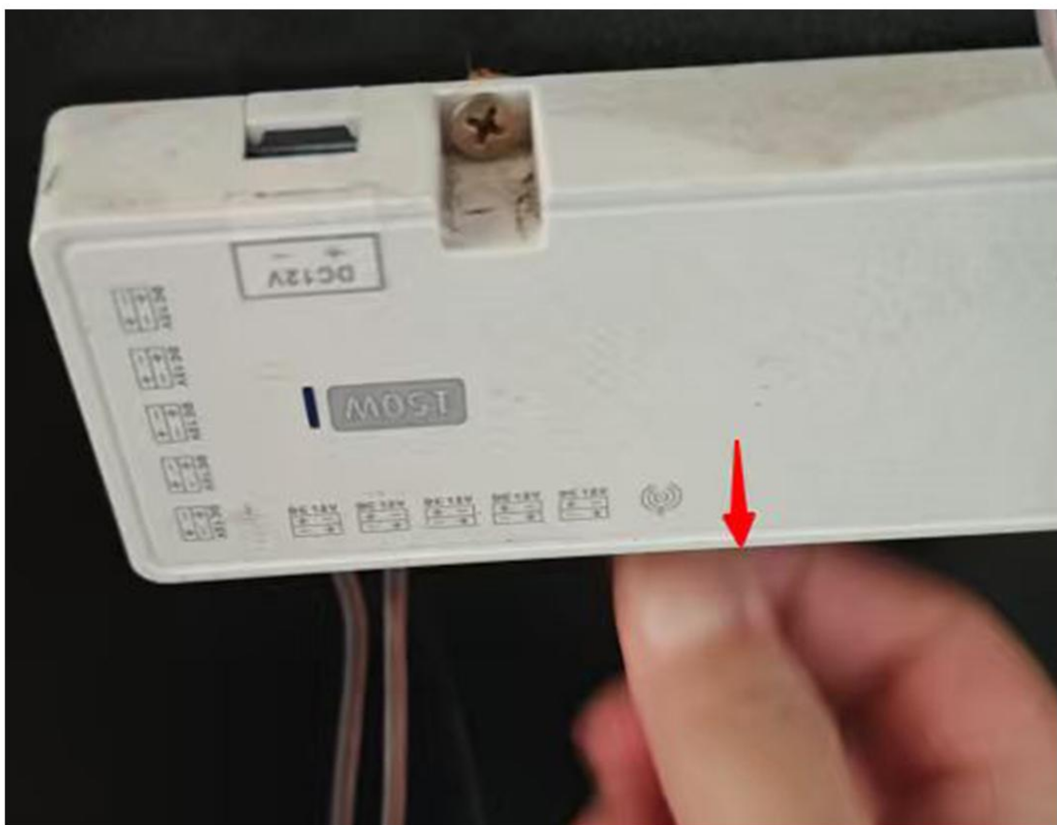
Step 2: Unplug the power cord of the original switch.
