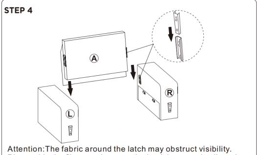
Please tidy the fibers and ensure the latch is properly aligned
