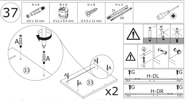
Install screw A on the wooden board 33, then connect the wooden board 33 to the wooden boards 34 and 35.
