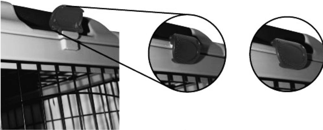
Step 12. Fasten latch on the left back cage as shown in Figure K. Repeat on right side.
