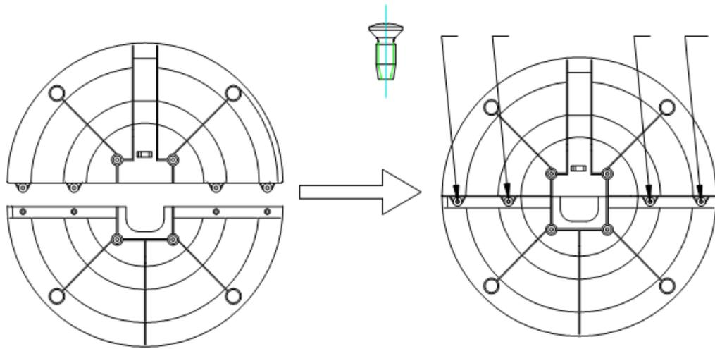
3. Pass the power cord through the bottom panel, and insert the base plate with four screws and the main body of the product.
