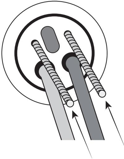
8. Put the water inlet pipe into the faucet hole of the counter, adjust the faucet to be in the correct position.
