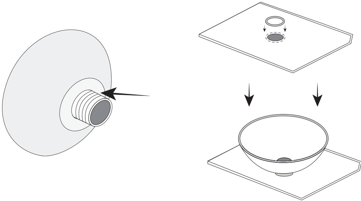
2. Put the rubber ring on the bottom half of the drain that is under the counter, then put on and tighten the nut.
