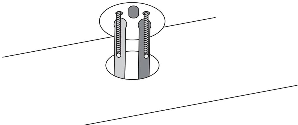
9. Adjust the direction of the faucet and install the U-shaped rubber pad around the bolts and water inlet pipes.
