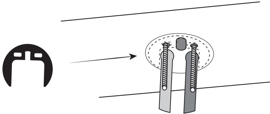
10. Install the U-shaped metal sheet and tighten the nuts onto the bolts to keep faucet in place. Ensure the faucet is secure. Attach included adapters to the end of the water supply lines, then connect to the building water supply line.
