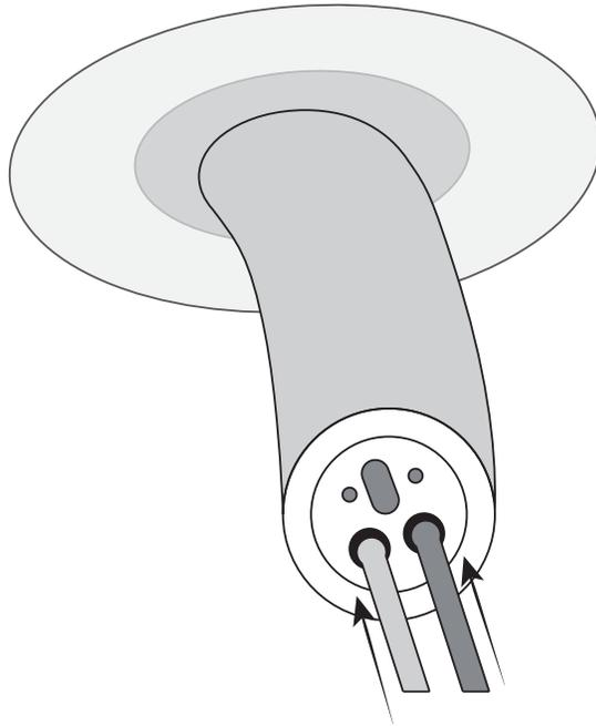
6. Put the small, round, rubber ring on the round edge of the indented curve.
