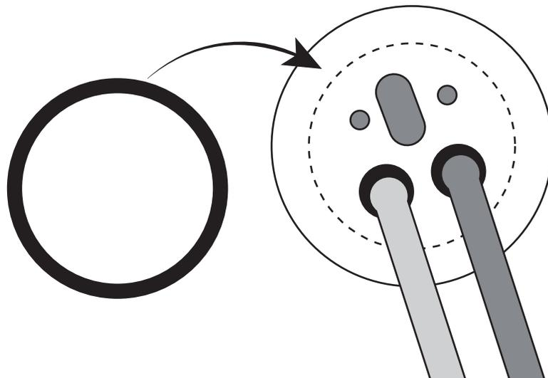
7. Screw in both bolts about a quarter of the way into the bottom of the faucet.
