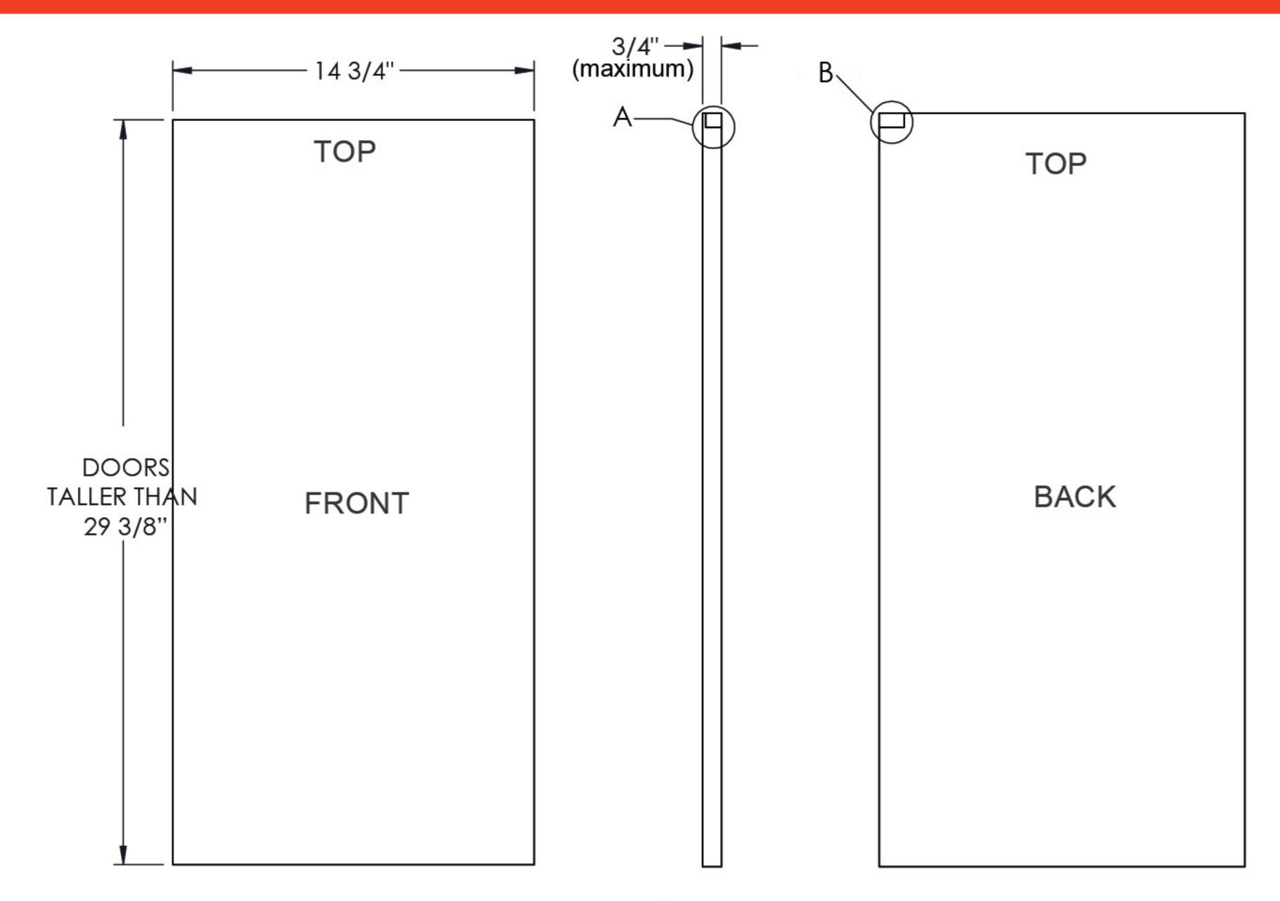
Door panels taller than 29 3/8" require a notch as seen in Detail A & B on the hinge side.
