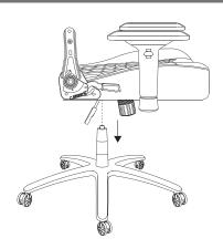
Align the hole in the Control Mechanism with the top of the Gas Lift Cylinder and push down firmly.
