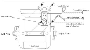
Remove (4) Set Screw and Washer Sets (Part L) from the underside of the Seat (Part B) and align the holes of the Control Mechanism (Part J) with the holes in the seat ensuring control lever is facing the Right Arm **and** Tension Knob faces the Seat Front. Tighten with Allen Wrench (Part N).
