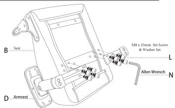
Remove (8) Set Screw and Washer Sets (Part L) from the underside of the Seat (Part B) and align the holes of the Armrests (Part D) with the holes in the seat. Tighten with Allen Wrench (Part N).
