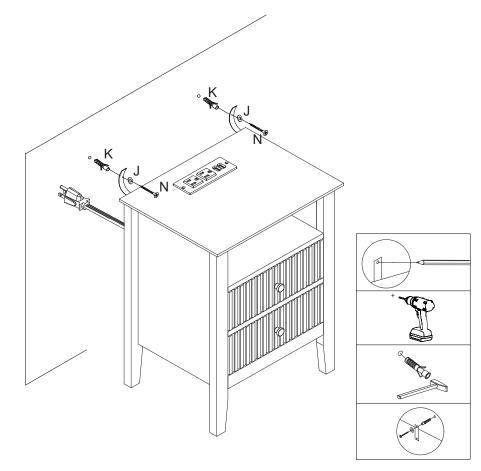
Use components K, J, and N to assemble hardware L on the wall to prevent tipping.
