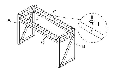
3 Attach the frames (E) to the left & right leg (A & B) and cross bar (D). Using bolts (H) and L-allen key (J) to tighten.
