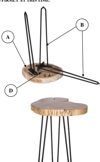
TIGHTEN ALL BOLTS FIRMLY AT THIS TIME USING ALLEN KEY (D). SET ROUNDEND TABLE UPRIGHT.
