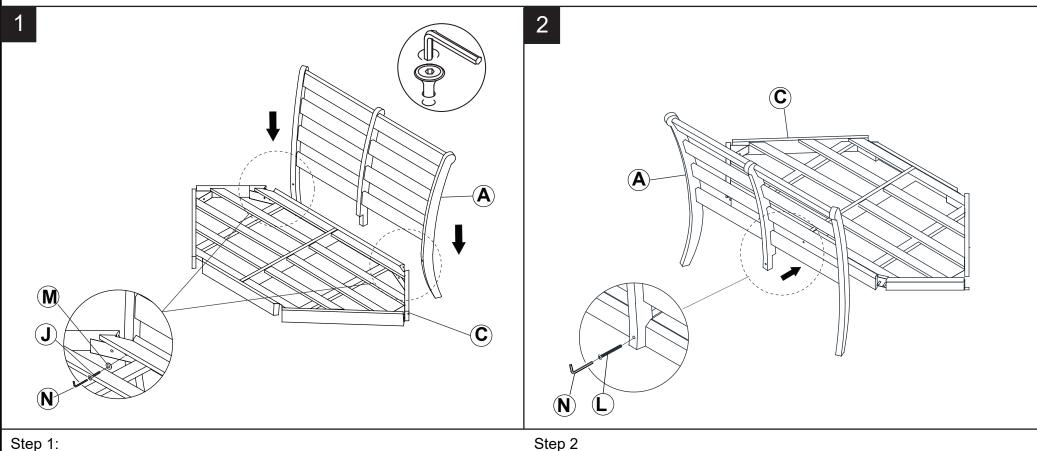
Attach Frame Back 1 (A) to Frame Seat (C) ,use Bolt (J) and Washer (M) tighten with allen key (N).
