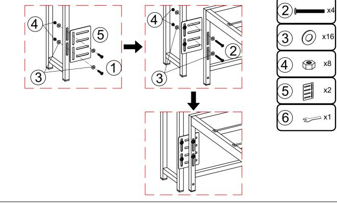
When the installation distance between the headboard bracket and the bed frame (not included) is just fine, an adjustable board can alsao be used to link.
