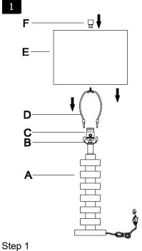
Insert the Harp (D) into the Saddle (B). Put the shade(E) on the Harp(D), then tighten the Finial (F) into the Harp (D)
