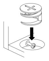
Turn cam lock clockwise to tighten.
