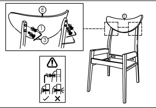
Place the Top Rest (E) on the back frame as shown above.
