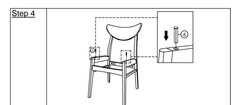
Place Wood Dowel 6 on the Side Frame as shown above.
