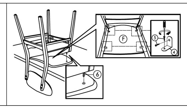
Place **the Cushion Seat(F)** on the table, then put the assembled chair parts in Step4 to fix the Cushion Seat (F) as shown.
