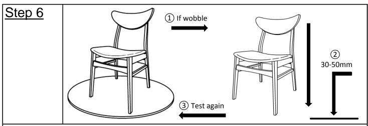
Place the dining chair on a Level Surface to check if it wobbles. loosen the bolts. lift the dining chair some 30cm to 50cm high from the ground, keep your feet and toes well away from the drop zone, and drop the dining chair freely and vertically with the four legs, hitting the ground at the same time. This Drop Test will help to ensure that all the bolts and gaps to all reach full alignment.
