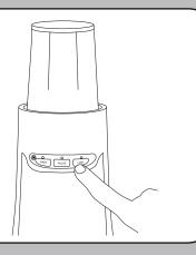
Lift the cup from the base, unscrew the blade assembly and empty the ingredients.
