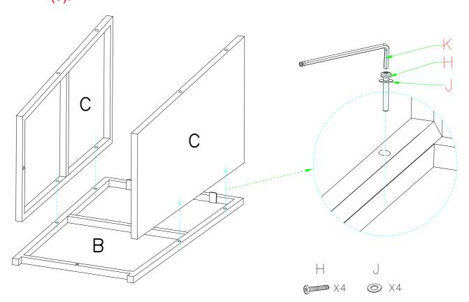
**Step 2.** Attach Bottom Panel (D) to Side Panel (C) and Front Panel (B) using a Long Bolt (H) and Flat Washer (J).
