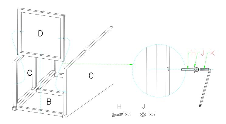
**Step 3.** Attach Back Panel (A) to Side Panels (C) and Bottom Panel (D) using a Long Bolt (H) and Flat Washer (J).
