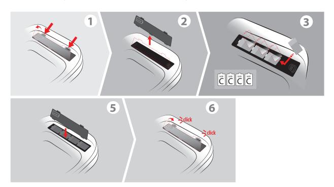
A set of 4 new Alkaline C-sized batteries can can last up to a year. AC adapter is optional and can be purchased separately at www.itouchless.com/parts.
