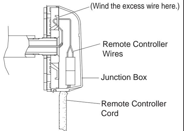
3. Insert the wall pipe containing the remote controller wires through the hole.
