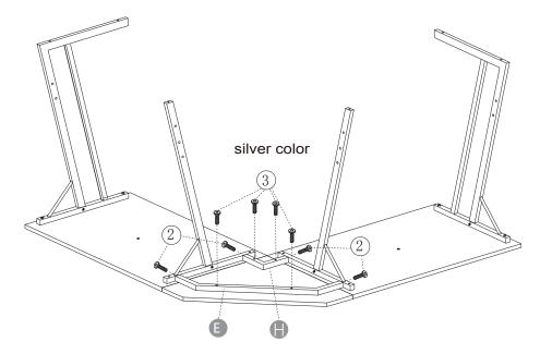
Notice: Fix the No. 2 screws firstly, then assemble the No. 3 screws.
