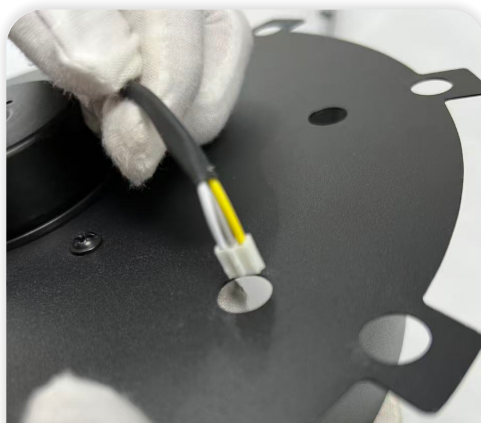
7 Pass the lamp holder wire through the base screw hole.
