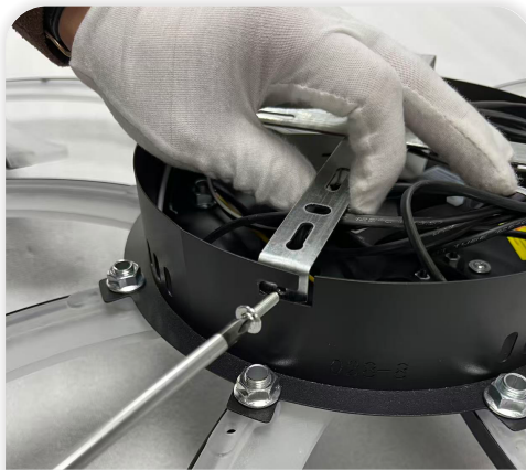
20 Lock the side screws of the base.
