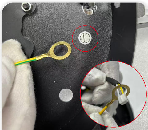
10 Locate the hole marked for the ground wire.
