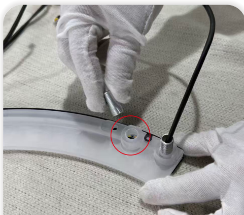
4 Tighten the nipple screw.
