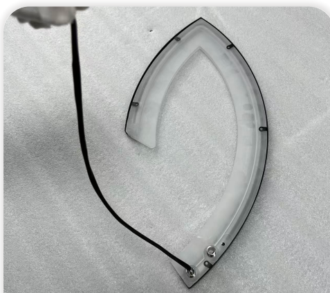
5 One lamp holder is installed.
