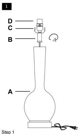
Pull power cord to connect the Neck (B) to the Base (A).
