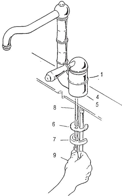
Under the sink, stack the half ring rubber gasket - 6, the half ring mounting plate - 7, then the mounting nut -9 onto the stud.
