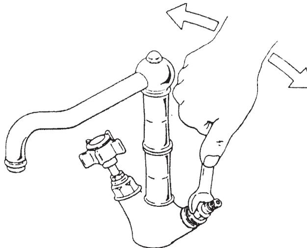
3. Remove the cartridge with a smooth jawed wrench or 17mm wrench
