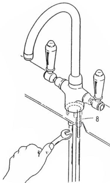
5. Check the position on the sink of the faucet, then tighten the nut with a 13mm wrench.
