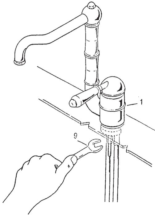
Check the position on the sink of the faucet, then tighten the nut with a 13mm wrench.
