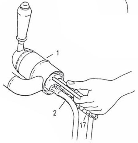
Install mounting stud securely or verify it is installed.
