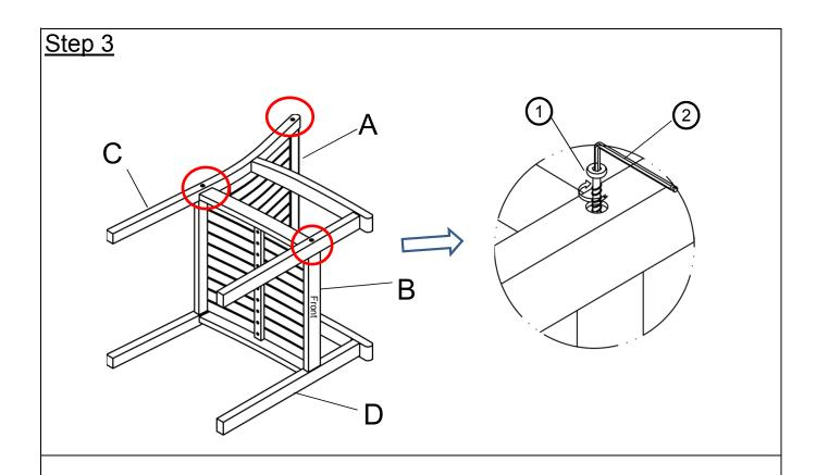
With assistance from an adult partner, turn the Chair Frame over onto the other side. Attach First Leg Panel(C) to Backrest Panel(A), and Seat Panel(B) using Screws(1) with Allen Key(2).
