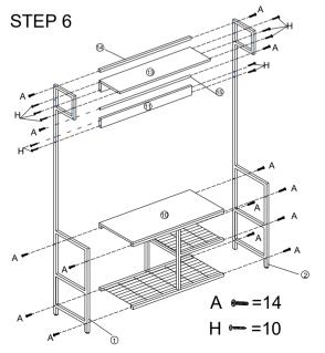
As shown in the figure, connect them with screws A and H.
