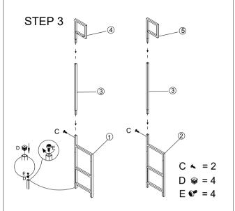
Install D and E at the bottom of NO. 1 and NO.2. Insert NO.4 and NO.3 into NO.1 in sequence, and then insert NO.5 and NO.3 into NO.1 in sequence. And fix No. 1 and No. 3, as well as No. 2 and No. 3, with screw C.
