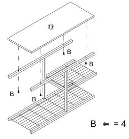
Use screw B to connect No. 10 to the frame.
