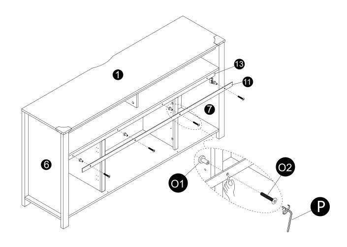
· Attach part (11) to panel (13) with parts (O) correctly.
