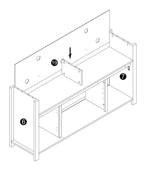
·Carefully slide panel (19) into place along the back of the assembly.
