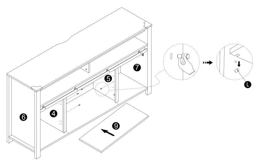
· Attach panel (9) to panels (4,5) using parts (L).
